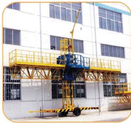
单立柱 (Single Mast climbing working platform)
